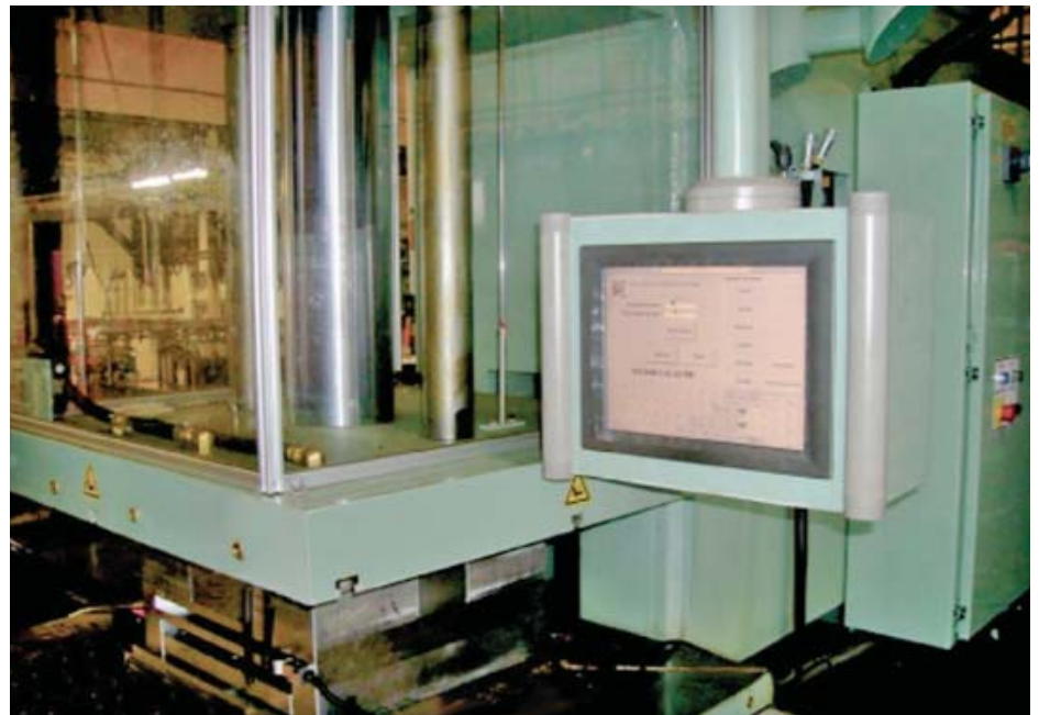
MPI's Touch Screen Smart Controls, running the Guardian Foundry System.
